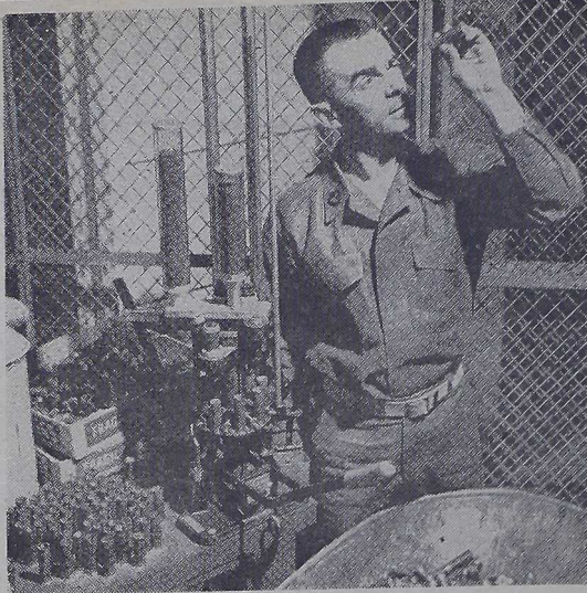
AMMO MAKER —Act. GySgt. Tony Meniz inspects an empty shotgun shell casing before placing it on the assembly line that produces skeet range ammunition. The NCO-in-charge of the Base Skeet Range says the vertical tubes on the machine contain lead shot pellets, gun powder, filler wads, over-powder wads, and primers. One complete shell is made every time the lever at the base of the machine is pushed up. (Photo by Act. Sgt. J. E. Horecka)
