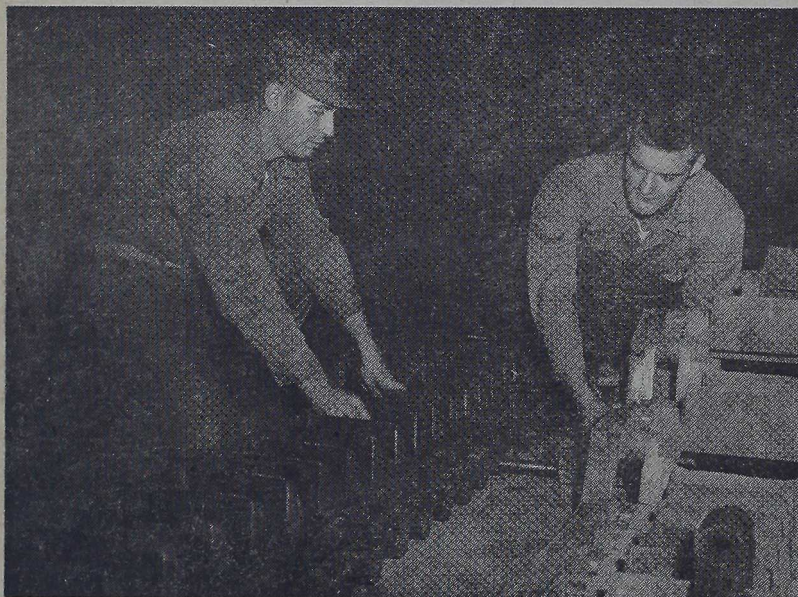
TRACK REPAIR —Act. Cpl. H. Drake, left, and Pfc J. S. Saladin, H&S Co., 2nd AmTrac Bn., repair and replace worn-out and damaged tracks as part
