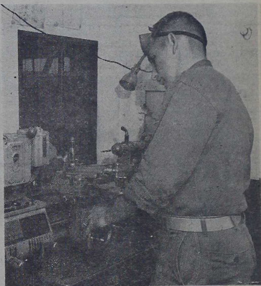
PARTS MANUFACTURE —Making a loading ramp pin for an LVT P-5 is Act. Sgt. Gerald Schimpf, H&S Co. The mobile machine shop where Sergeant Schimpf is working is used for the manufacture of small parts and is also equipped to assist during field operations.
