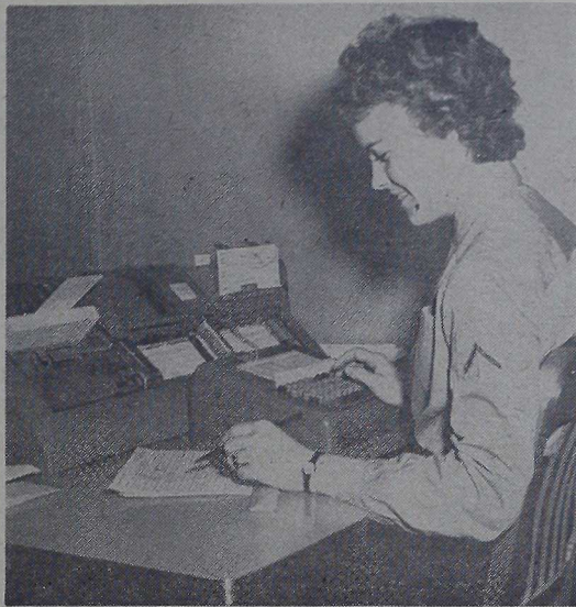
VERIFIER —Pfc Shirley A. Smitherman, Key Punch Verifier Machine Operator, verifies information punched on cards by the key punch machine. All information punched on the key punch cards must be checked by the verifier machine.
