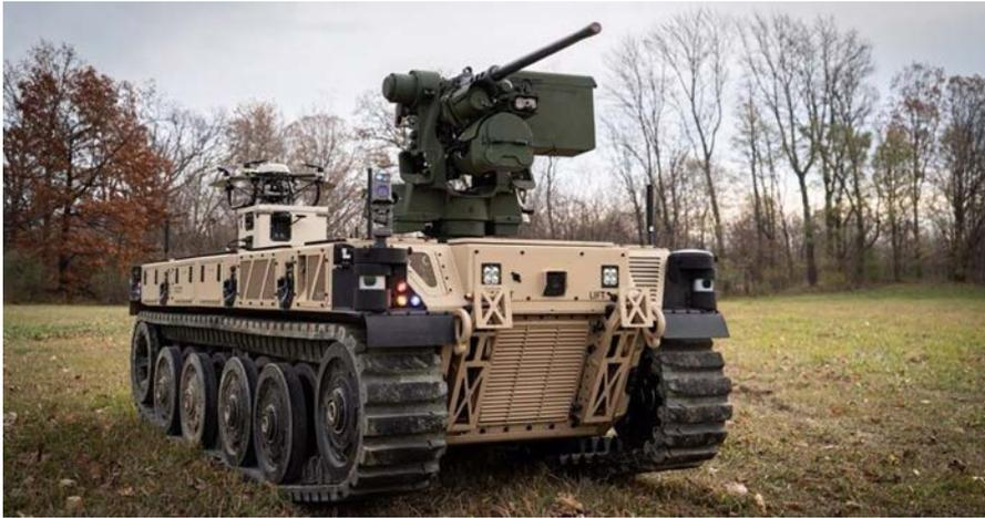
**Figure 1. The RCV-Light can be equipped with a tethered unmanned aerial system, a small drone that can be deployed to conduct aerial reconnaissance while the vehicle is at a safe distance. Other equipment to be tested on the RCV-Light experimental prototype includes the M153 Common Remotely Operated Weapons Station II (CROWS II), the .50 caliber M2 machinegun and the 40mm MK19 Mod 3 automatic grenade launcher. (Photo by Bruce Huffman, Michigan National Guard)**
