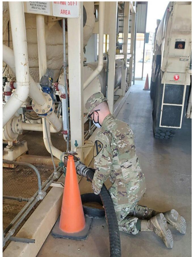
**Figure 7.** A Pegasus Harvest maintenance Soldier purges an M-978A2 Heavy Expanded Mobility Tactical Truck at a purge site. (U.S. Army photo)
