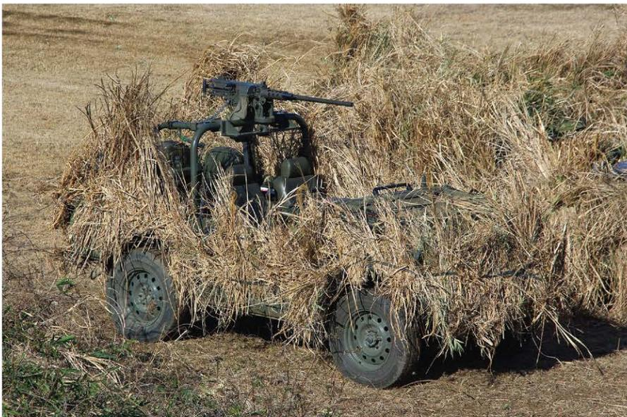
**Figure 4.** An example of blending: a Japan Ground Self-Defense Force Type 73 Ougata light truck camouflaged into its surrounding background.
