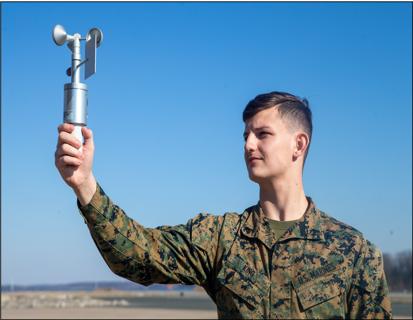
U.S. Marine Corps Cpl. Haydon R. King, a meteorology and oceanography analyst forecaster with Marine Corps Air Facilities Quantico reads the information off of an anemometer at Marine Corps Base Quantico, Virginia, Jan. 26. The anemometer is a weather instrument used to read both wind speed and direction.
