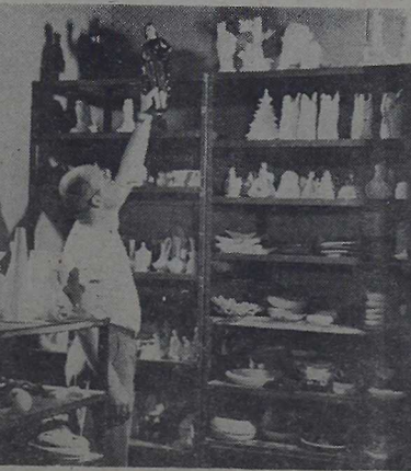
FINISHED PRODUCT—SSgt. Galen H. Moore, NCOIC of the Base Ceramics Shop, places a completed figurine on the shelf after firing, the process which bakes the glaze at temperature of 1,873 degrees.
