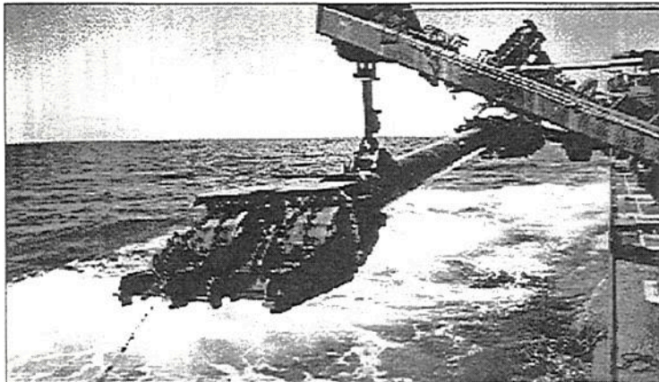
Raising a dragarm lifts its huge draghead out of the water. Acting as a marine vacuum cleaner, the dredge picks up sand and silt from the floor of the bay.
