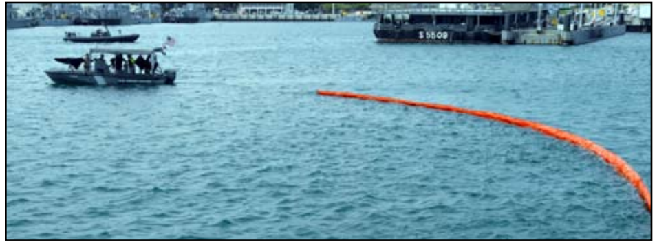
A 25 foot Transportable Port Security Boat manned by Coast Guardsmen from PSU 301 who will soon redeploy back to the U.S. and some of their replacements from PSU 312 guide the boom into place which would keep the oil spill floating on the water from spreading until it can be removed.
