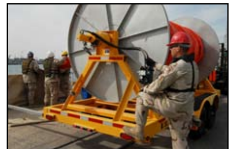
Petty Officer 1st Class Carl M. Sette, machinery technician, Port Security Unit 312, operates the hydraulic control on the oil containment boom to regulate the rate the boom is played out Dec. 14.
