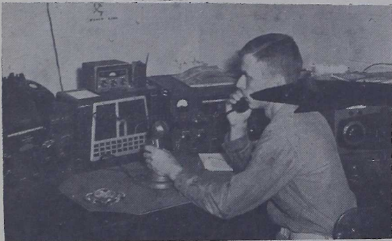
HELLO, GUANTANAMO. THIS IS LEJEUNE —Cpl. William Markwood, radio operator at the Base Amateur Station, makes contact with a station in the Caribbean before setting up radio-telephone communications with a Lejeune-based Marine and his family residing in the Jacksonville, N. C., area. The connection is made by an instrument called a "phone patch" to both transmitter and telephone at the station. (Photo by Cpl. S. P. Rice)
