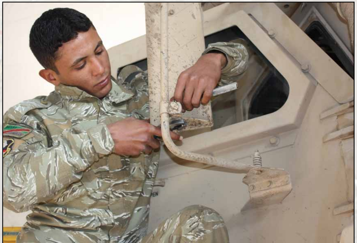
Using a ratchet and a wrench, Pvt. Ali Kitab Sarhan, 11th Iraqi Army, tightens the bracket that holds the rearview mirror in place on their vehicle while attending a maintenance class, at Victory Base Complex Jan. 7.
