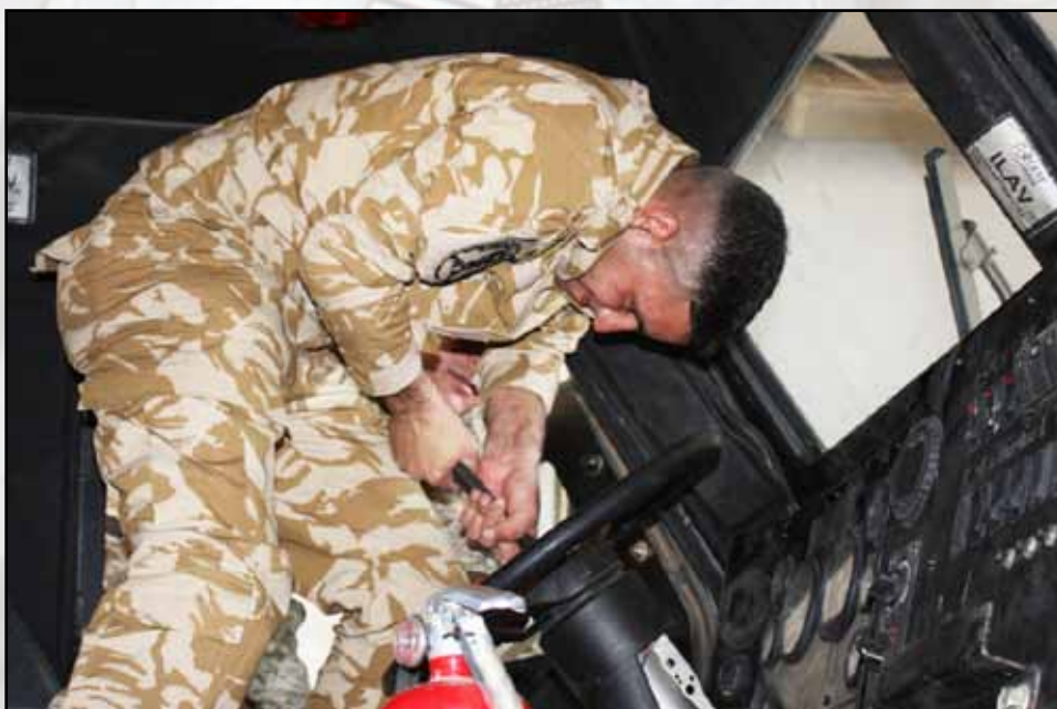
Using an adjustable wrench for the first time, Pvt. Hayder Maky, 11th Iraqi Army, tightens the steering column to their Badger, an Iraqi light armored vehicle, at Victory Base Complex Jan. 7. Six Soldiers from the 11th IA attended a three-day Badger maintenance course covering basic repairs and tool familiarization.
