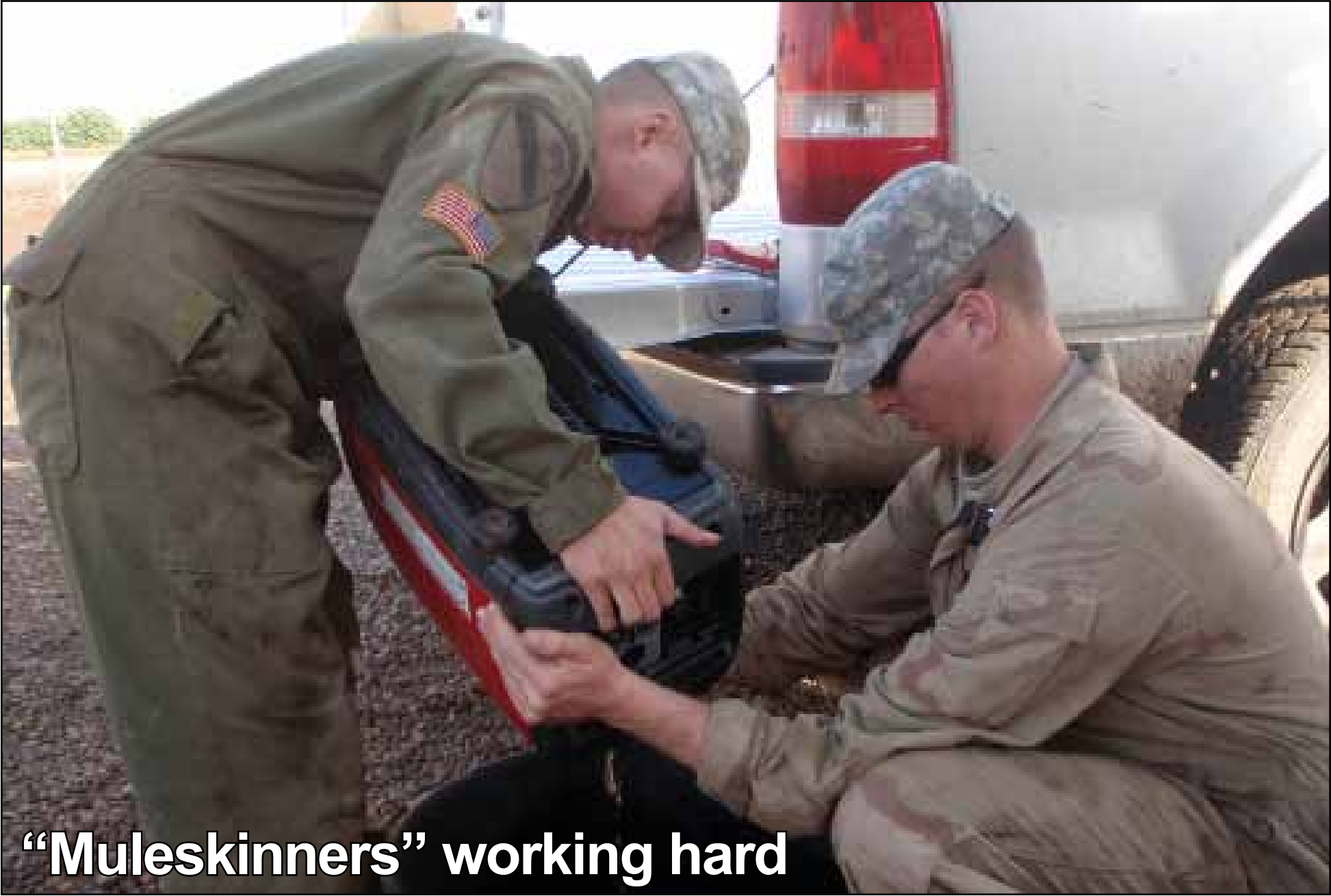
CAMP TAJI, Iraq – Beemer, Neb., native Spc. Devon Pagels (left) and Issaquah, Wash., native Spc. Brenton Nikolaus, both wheeled-vehicle mechanics assigned to Company B, 115th Brigade Support Battalion, 1st Brigade Combat Team, 1st Cavalry Division, drain fluids out of a generator at Camp Taji Jan. 5.
