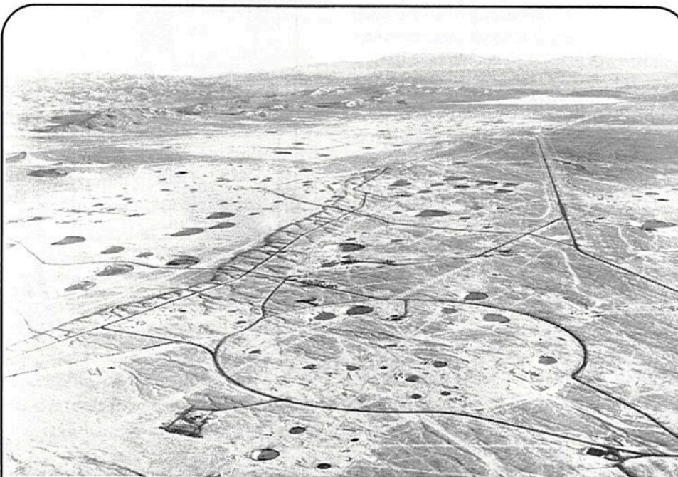
NF-474 Most subsidences leave saucer-shaped craters varying in diameter and depth, depending upon the yield, depth of burial, and geology. This is the north end of Yucca Flat. Most tests are now conducted in this valley.
