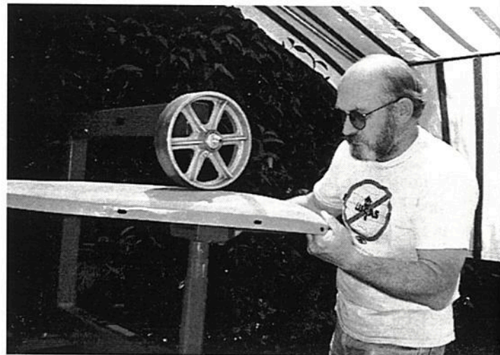
Watt hard a work "wheeling out" the right curvature on a Triumph rear fender, with an English Wheel.
