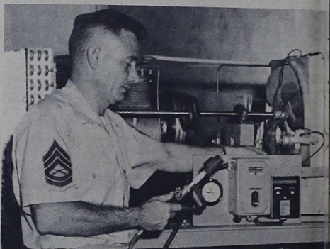
NEW TRAINING AID —GySgt. Reno R. Renaldo, refrigeration instructor at the Utilities School, Marine Corps Engineer Schools, demonstrates the checking procedure for leaks, using acetylene, on the "exploded" model of the Refrigeration Unit which he designed and constructed from salvaged parts for instructional purposes. (Photo by B. J. Martin).
