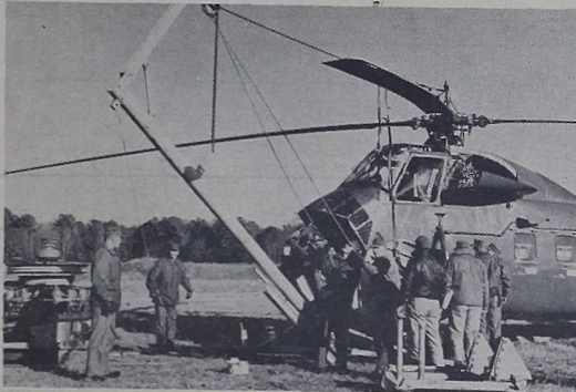
CHANGE IN THE FIELD —Members of Headquarters & Maintenance Squadron-26, MAG-26, MCAF New River, use the expeditionary maintenance hoist to change the engine of a downed helicopter in a tobacco field near Tarboro. The pilot of the helicopter, Lt. Col. C. L. Champion, who developed the hoist being used, was flying from his home base of MCS Quantico to Jacksonville, Fla., via New River.
