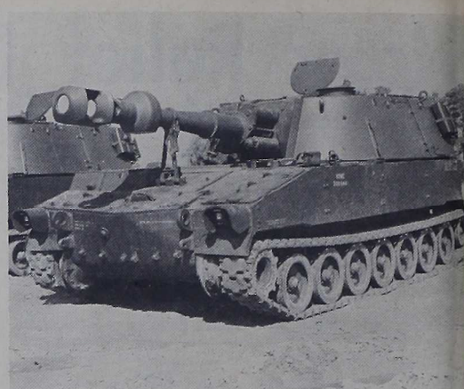
NEW 2D DIVISION SUPPORT —The M109, a new 2d Marine Division supporting arms weapon, is self-propelled, armored and mounts a 155mm howitzer on its turret. Highly mobile, the 26-ton artillery weapon can blast target at ranges of 18,000 meters.
