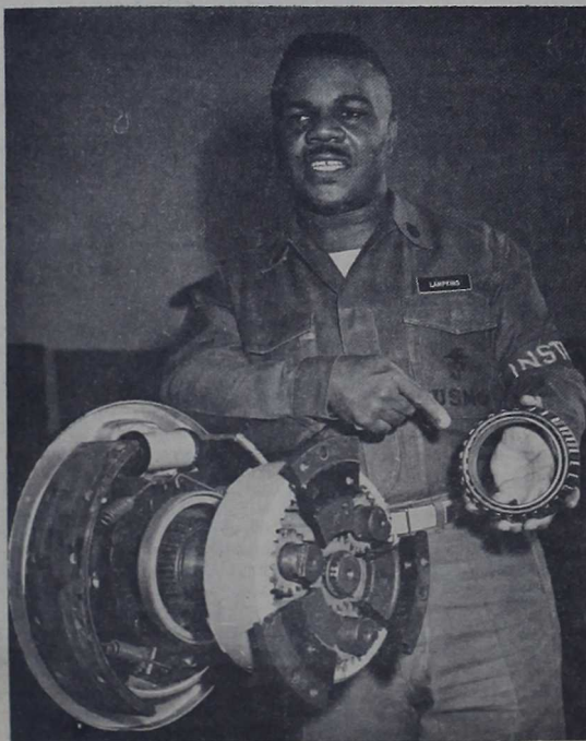
THE PRIDE AND JOY of SSgt. O'Larry Lampkins is this cut-a-way, yet moveable, visual training aid used in the instructions on the standard axle. The cutting and painting required to complete this aid consumed nearly 80 hours of Sgt. Lampkins personal time.
