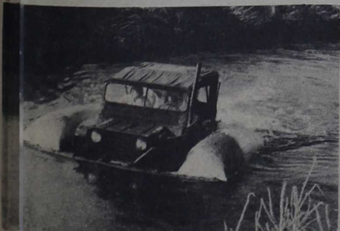
AMPHIBIOUS QUARTER-TON —The driver of this vehicle becomes a pilot when the water wings are used for floating along in deep water. Rubberized nylon bags are inflated with exhaust gases from its motor and the floating vehicle is propelled by the action of its wheels in the water. This new type swimmer is being tested for possible military use.
