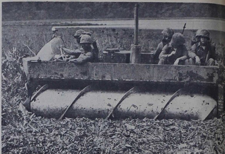
ONE OF MANY new items of equipment that the Marine Corps Landing Force Development Center takes a look at each year in an effort to find the right equipment for the fighting Marine is this amphibian called the Marsh Screw. This vehicle was recently evaluated for
