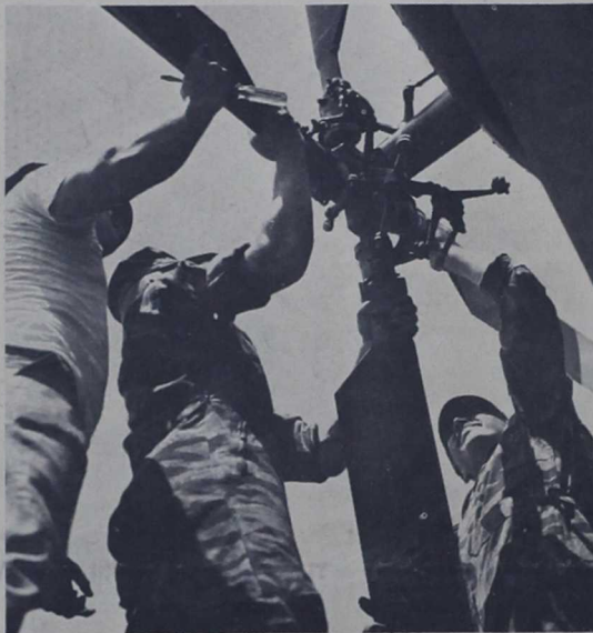
SLIGHT ADJUSTMENT —To make an adjustment in the rotor head on the tail section of a UH-34D helicopter, (left to right) PFC Albert P. Montell, Cpl. Edward D. Briscoe and Cpl. Gary L. O'Neill find it necessary to remove the rotor blade.
