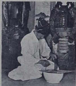
ANCIENT PROCESS —Using a process thousands of years old, Mr. Kunitoshi Fujimura coats a blade with a clay mixture prior to tempering. Mr. Fujimura, who has been a swordsmith for 30 years, wears the traditional robes of his trade.
