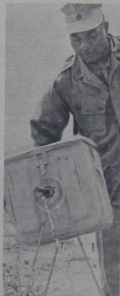
FRESH OFF THE ASSEMBLY LINE -- SSgt. Walter Mothershed (Elsinor, Calif.), a platoon sergeant with 1st Bn., Twelfth Marines, demonstrates his improvised washing machine. The main body of the "Mothershed Machine" is a steel box which once held 12 time fuzes. Ammunition rods serve as legs for the washer and ammo boxes make up the base. Steel rods welded on each side act as handles to turn the box and agitate the clothes. (Photo by PFC G. R. Durbin.)
