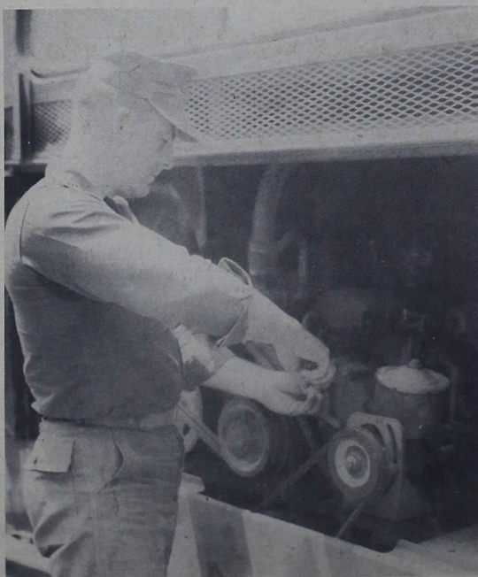
A WATER HOSE is tightened by Sergeant Jerry A. Bell, mechanic, on a huge diesel bus engine. Preventive maintenance such as this must be performed everyday.
