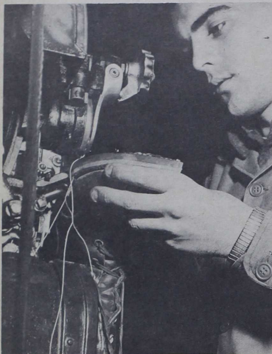
COMBAT COBBLER — Applying the stitches to the sole, "combat cobbler" practices his trade utilizing modern field transportable machinery. (photo by Cpl. J. T. Fredd)
