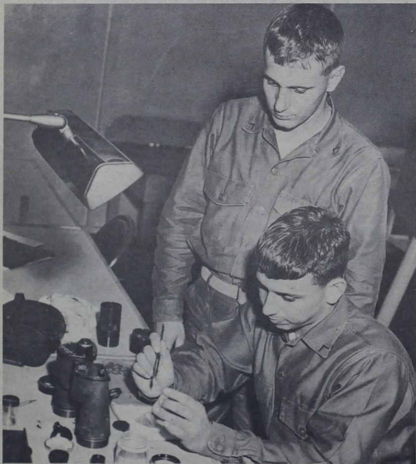
POLISHING the delicate lens from a pair of binoculars — From delicate optics to over-
