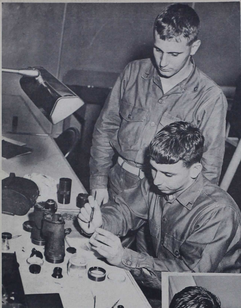
POLISHING the delicate lens from a pair of binoculars—From delicate optics to overhauling tanks Maintenance Battalion is there to repair.
