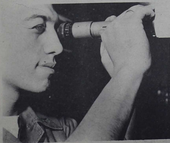
ONE EYE CLOSED , a "sight mechanic" makes good use of the other adjusting the sight aperture of a 30 caliber machine-gun from an Amphibian Tractor. The sight aperture enables the "amtrac'ers" to sight and fire through a periscope.
