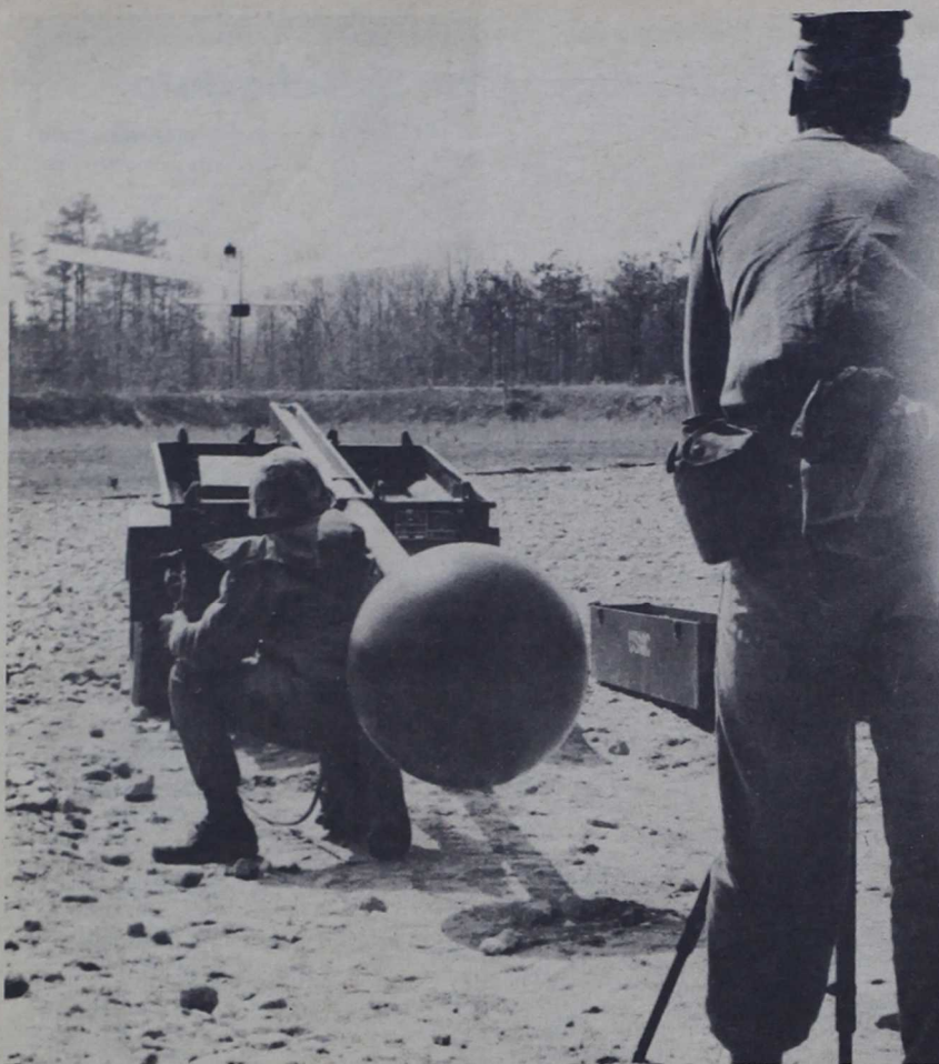
THE BIKINI DRONE, a remote controlled, self-propelled reconnaissance plane, complete with camera, is launched during the exercise. The drone, used by Company C, 2d Recon Battalion, was tested during the operation.
