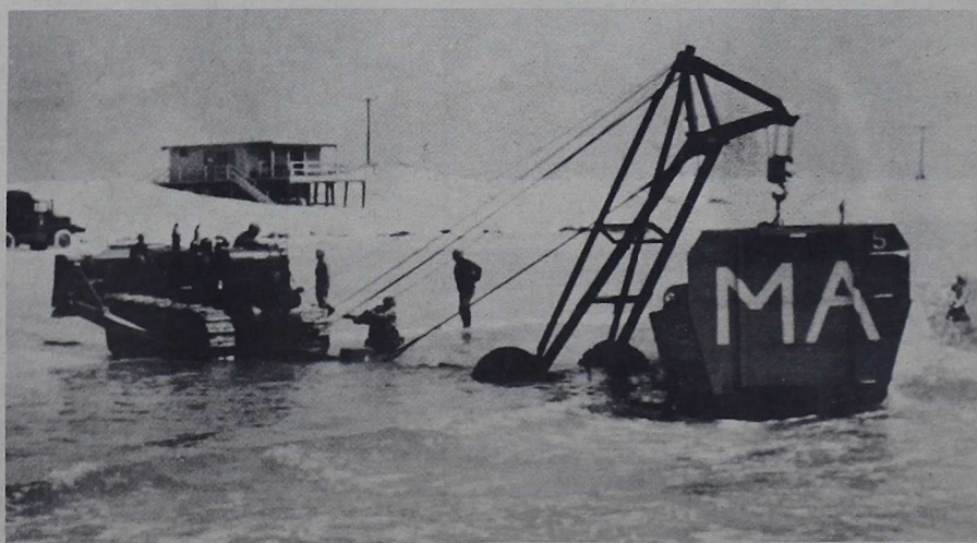
IN TROUBLE — Members of the Salvage Section, Naval Beach Group, part of a Shore Party Team when task organized, use a TD24 and Surf Crane to lift a disabled Peter Boat out of the water for repairs.
