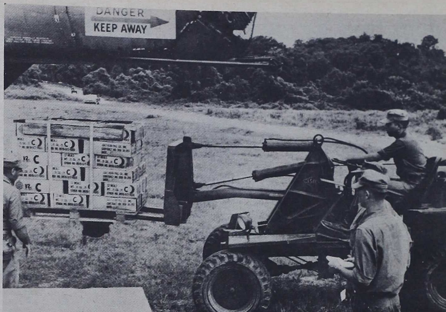
A BIG LIFT — A 3000 lb. fork lift is used to unload a pallet of sea rations from a helicopter during helicopter-borne landings recently. Men from Shore Party form the nucleus of Helicopter Support Teams used in unloading supplies during such operations.
