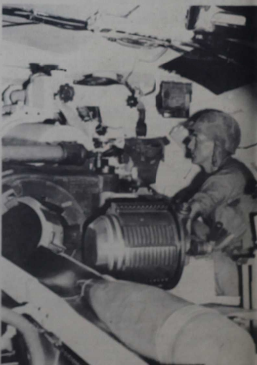
LOCK AND LOAD... 300 pounds of powerful explosive stand ready to be fed automatically into the breech upon the command from the Fire Directional Control center.
