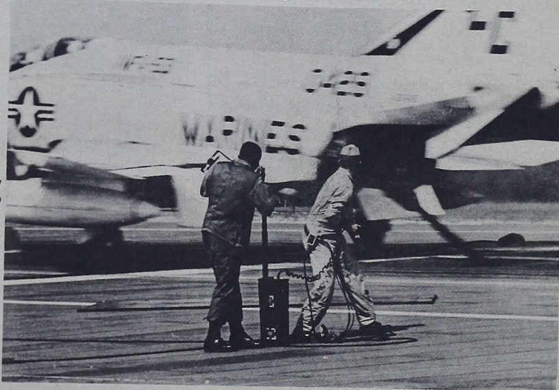
AN ARREST IS MADE - Line crewmen insure that the F-4 is properly arrested as its tail hook connects with the short distance stopping cable.
