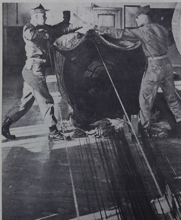
CLEARING A PARACHUTE -- Members of the Air Delivery Platoon use a large fan to clear a cargo parachute in preparation for packing. The long shroud lines must be untangled and straightened before beginning to re-pack a parachute.
