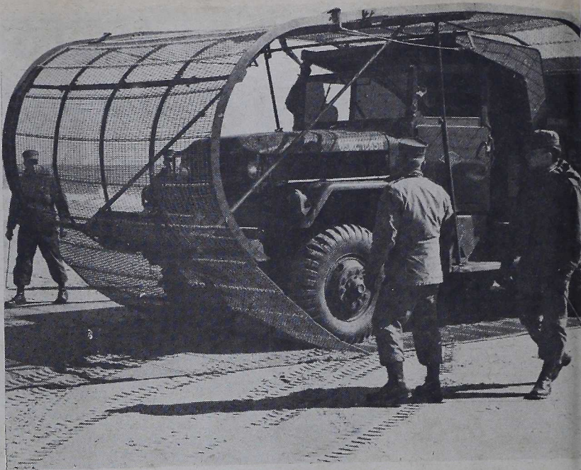
ROLLING OUT THE CARPET - The M 51 Mat Laying vehicle unrolls its metal carpet to the landing craft to facilitate off-loading of heavy vehicles on the sandy beach.
