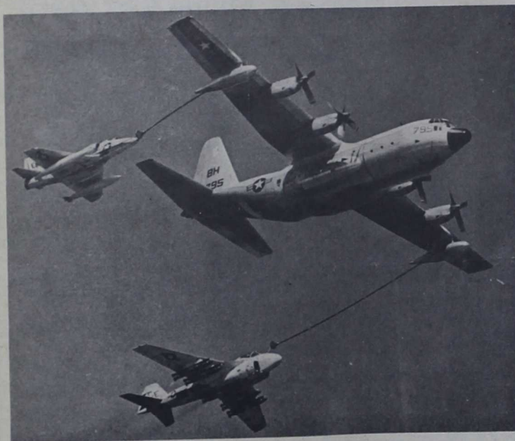
A C-130 HERCULES refuels a A4D Skyhawk (upper left) and a A6A Intruder (lower left) during the ariel display at Bogue Field.
