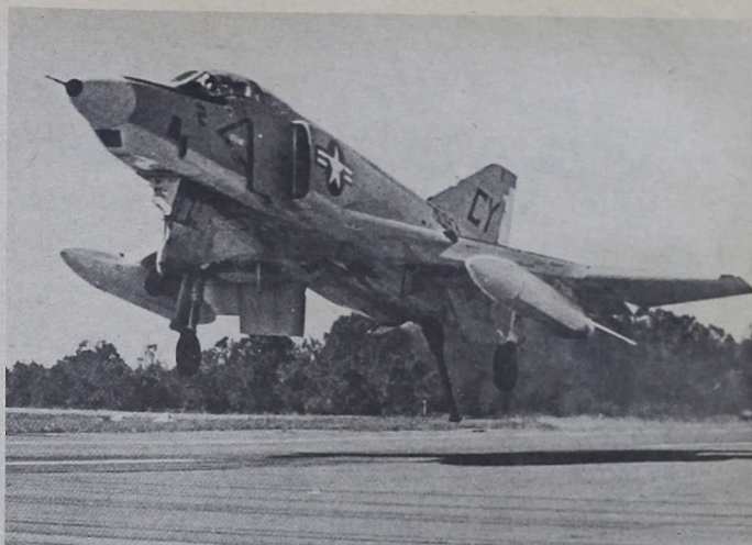
AN F-4 PHANTOM prepares to demonstrate its ability to come to a complete stop within 300 feet after picking up the arresting cable with its tail hook.
