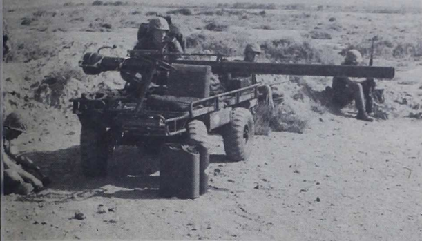
ANK KILLING 106mm recoilless rifle, attached to a "mule" zeroes in on prospective target on the beach. The sturdy little vehicle can carry 1,000 lbs 15 miles over almost any kind of terrain.
