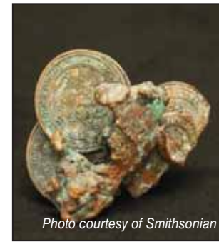
A pile of military challenge coins that were fused together by extreme heat from the hijacked American Airlines Flight 77 on Sept. 11, 2001.
