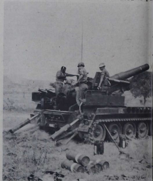
"ON THE WAY," a round from the M-110 self-propelled 8-inch howitzer will hit a target as far as 11 miles. The 204 pound high explosive projectile sounds like a freight train as it soars overhead.
