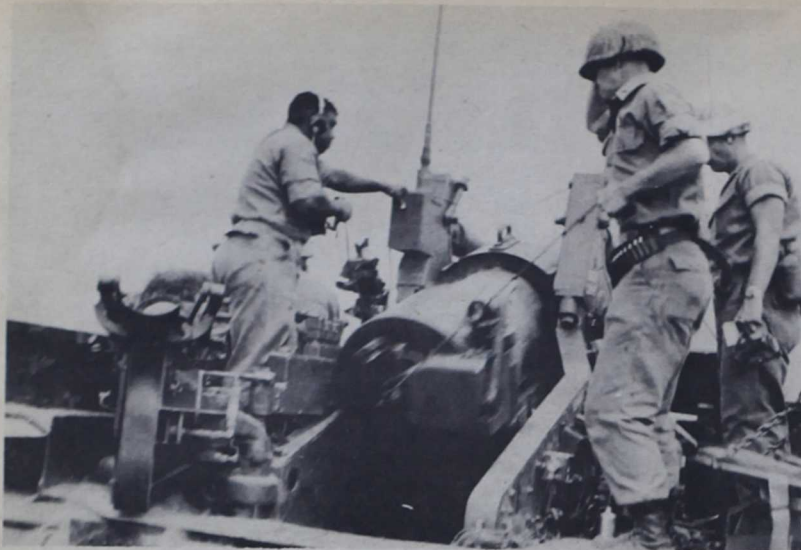
GUN CREW of the M-110 prepare to fire their giant artillery weapon. The crewman on the right wears a cartridge belt of primer shells used to fire the powder charge.
