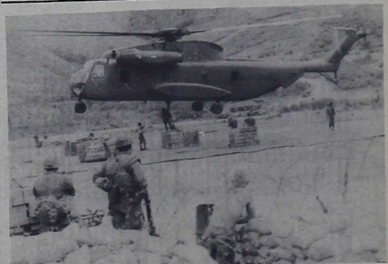
MARINES OF the 3rd Shore Party Detachment at Vandegrift Combat Base, 17 miles west of the Quang Trang Base, direct a heavy hauler Sea Stallion Marine helicopter over its external supply load while the hook-up is made.
