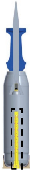
The first 120 mm cartridges qualified with the M125 thin-walled body primer in 1984. (Image courtesy of the author)
