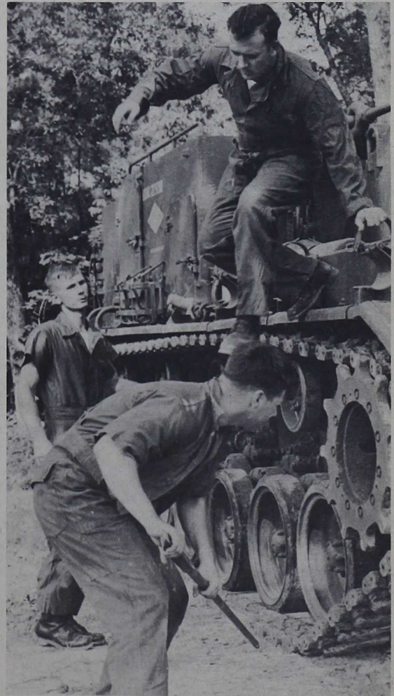
SERGEANT PAT BIANCHINI (atop vehicle), Sergeant Jerry Lynch (with crowbar) and Corporal Robert Malin get ready to repair track disengaged from sprocket of retriever. (Photo By LCpl. Don Abood)
