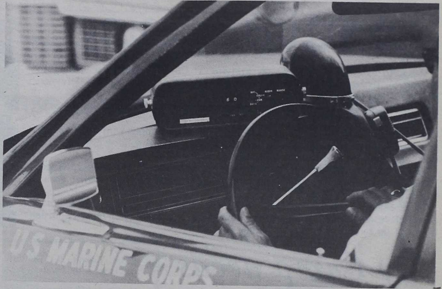
GET 'EM MOVING — A Military Policeman watches the control computer of an MR-7, mounted on the dashboard. He can spot speeding cars in oncoming traffic and vehicles to his front and rear.
