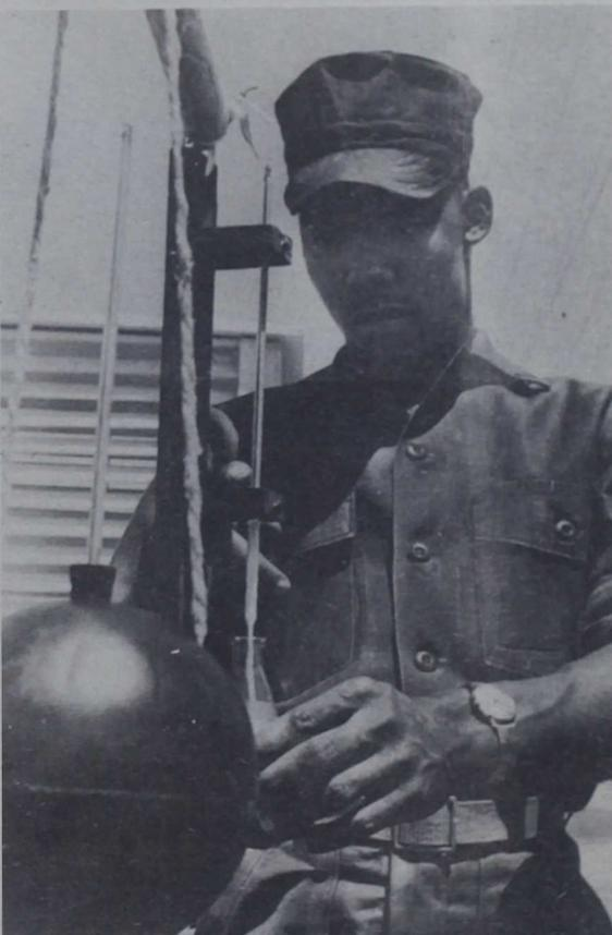
**LIFE SAVING STATION** — PFC William B. Richardson Jr., Training Facilities Div., Service Co., H&S Bn., takes the temperature from a natural wet bulb. This reading, along with those from a globe thermal and dry bulb will make up the correct wet bulb-globe temperature reading and determine what type of physical training is safe to conduct.
