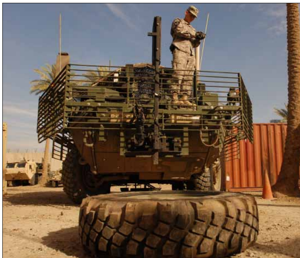
Spc. Robert Riddle, from Dallas, Texas, slides a new tire under the slat armor of a Stryker in order to change a tire on the vehicle, at Joint Security Station Justice, Dec. 18.
