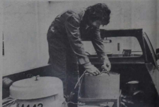
SMOKIN' JOE — Frank R. Encolanese, pest control operator, Insect Vector Control, makes sure he has a full container of insecticide before taking "Smokin' Joe," the ULV (ultra low volume) truck-mounted insect sprayer, to the field.
