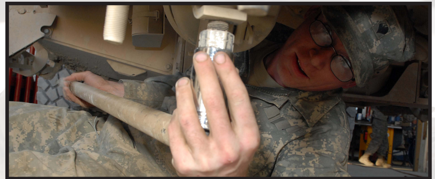
Army Spc. Thorsen Shoupe, a mechanic for mechanic platoon, G Co., 725th Support Battalion, removes the bolts of near a leaf spring of a Mine Resistant, Ambush Protected vehicle on FOB Salerno, Afghanistan, Dec. 23.
