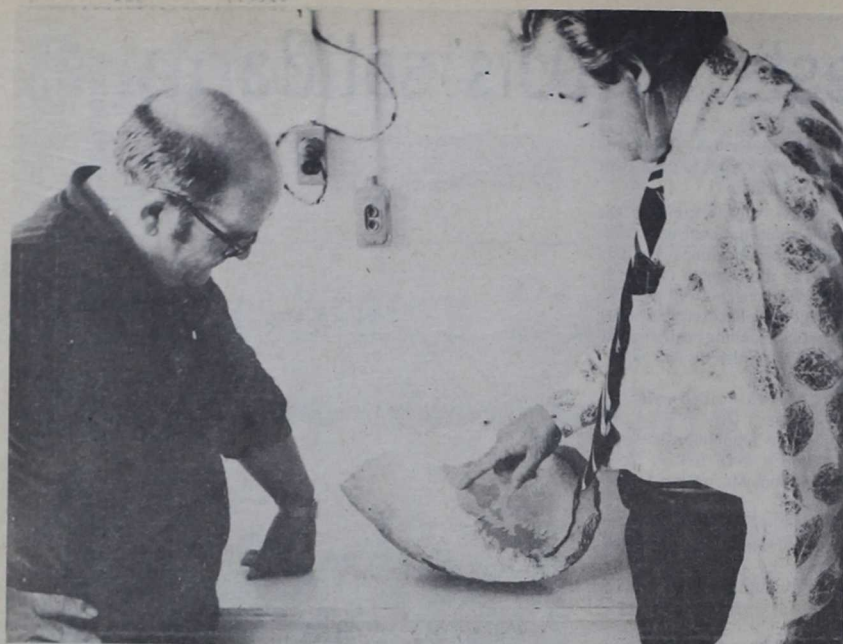
USED LIME — Willard R. Price (right), general foreman at the Hadnot Point Water Treatment Plant, points out various compound layers of calcium, iron, magnesium and lime deposits removed from a water treatment line to Stan A. Pehowic, a plant employee. Lime is used in the treatment process and filtered out of the water prior to the water leaving the plant. (USMC photo by SSgt. Arvel "J" Edward Hall)
