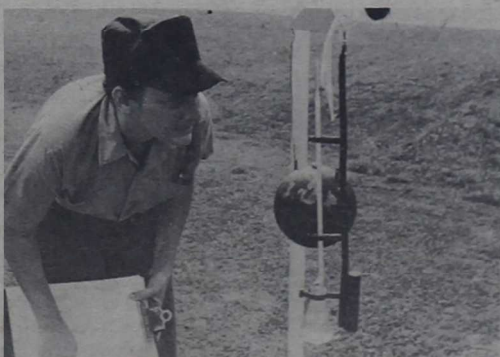
TEMPERATURE CHECK — Seaman Alita Beyers, a boat operator and wet bulb globe temperature (WBGT) index reader for the base training office, takes an hourly reading at the WBGT station, Bldg. 1404. The station is one of five located throughout Camp Lejeune, N.C. (USMC photo by SSgt. Brenda A. Lanclos)
