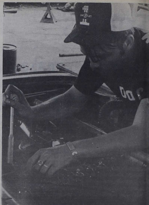
SURGEON'S HANDS — HM-3 Ken Barker adjusts the lifters of the McCary racing team's 6-cylinder engine.
