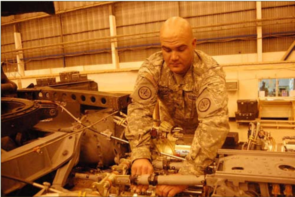
Spc. Donald A. Jackson, a Black Hawk Helicopter Repairer, inspects the main transmission oil filter on a UH-60A Black Hawk at the flight line. (US Army photo by Pfc. Jasmine N. Walthall)
