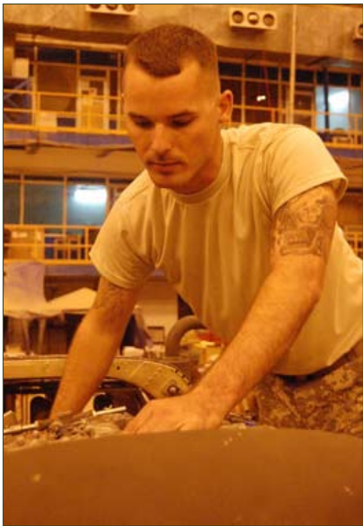
Spc. Thomas Spurgeon inspects the engine of an AH-64 Apache Helicopter. Spurgeon, a member of the 4th Squadron 3rd Armored Cavalry Regiment, inspects for and removes dirt and dust from the aircraft that may hide cracks or broken parts of the airframe. This routine maintenance is critical and helps ensure aircraft are fully operational. (US Army photo by Pfc. Jasmine N. Walthall)
