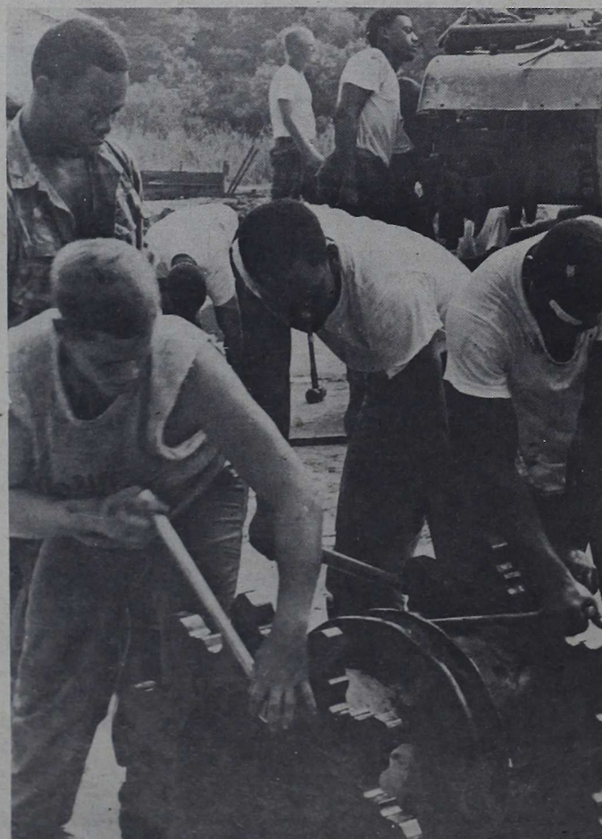
CHANGING SPROCKETS — Tank sprockets are the moving part of the vehicle's tracks. The sprockets rotate to lay and pick up the tracks, providing forward and backward movement.
