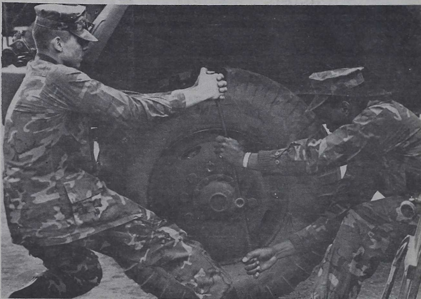
NUT CRACKER SWEAT — Working together, Pfc. Richard J. Long (left) and Pvt. Louis D. Rawles tighten lug bolts on a M54 five-ton truck. Both are Ground Specialty Orientation Program students from Truck Company, 8th Motor Transport Battalion, 2nd FSSG.
