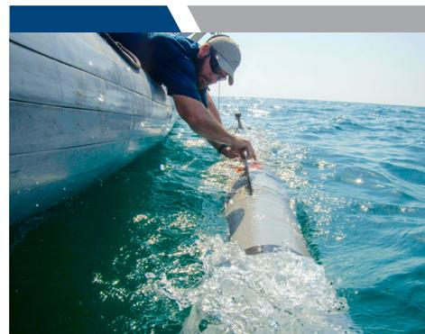
*An unmanned underwater vehicle (UUV) is deployed by an operator to search for possible objects of interest using side-scan sonar. A new partnership between NPS and Woods Hole Oceanographic Institution to create a virtual undersea environment could advance future UUV development, leading to an entirely new set of critical naval missions for these emerging systems. (U.S. Navy photo)*
