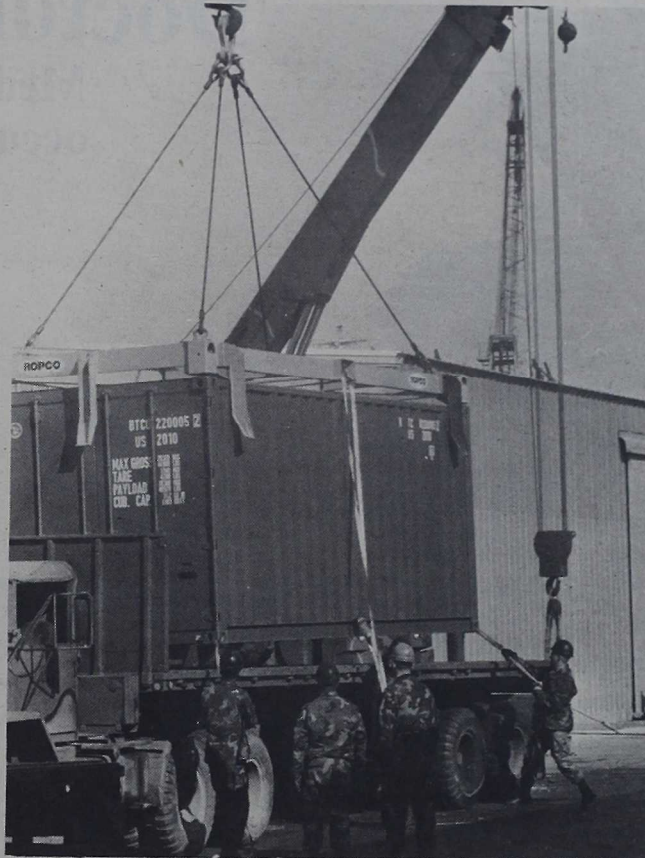
Marines make sure a cargo container is properly seated on a flatbed before being loaded aboard the Second Lieutenant John P. Bobo .
