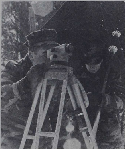
Corporal Dana Brown, instrumentman, aligns the sights of his automatic level for a field elevation reading, while Corporal Barbara Littell, recorder, records the data in her field notebook.
