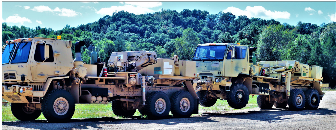
A military truck is connected to a military wrecker vehicle Sept. 23 as Soldiers at Fort McCoy for training in the Regional Training Site-Maintenance Wheeled-Vehicle Recovery Operations Course complete training at the installation Vehicle Recovery Site on North Post.
